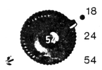
Nizo camera means that you can select the slow motion filming speed without the slightest delay when you need it. The black button in the center of filming speed switch 1 enables you to pass smoothly from 18 or 24 frames per second to 54 frames per second and back.
