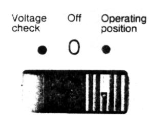
even if the camera motor is not run. For this reason, the master switch should always be turned to 0 whenever the camera is not operated a prolonged period. This will also prevent the camera from running if the shutter release is accidentally operated. Note, too, that if the handgrip is swung back but the master switch not set to 0, the meter battery will continue to operate at full power.
